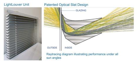
Figure 8: The LightLouver slat design.
