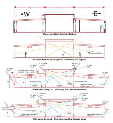
Figure 5: Iterations for controlling daylight within a class-room wing.
